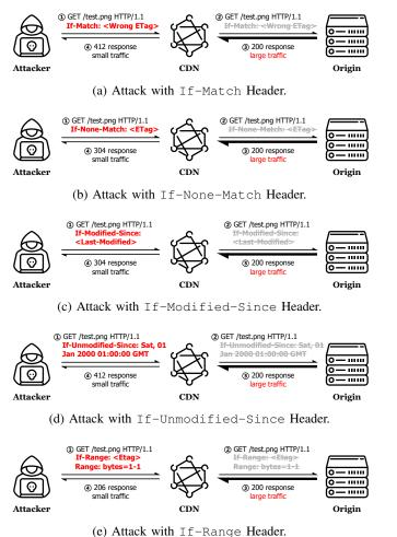
Fig. 10: Examples of CondAmp Attacks.
